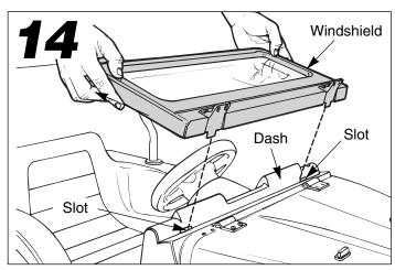
• Fit the tabs on the back of the windshield into the slots in the top of the dash.
